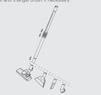
IV. Insert the handle to the larger tube end, and gently push the end to ensure firm locking. Use the tube in coordination with the crevice tool and triangle brush if peressary.
